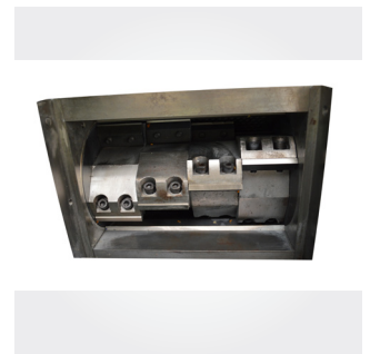
The staggered blades are angled to help improve efficiency.
