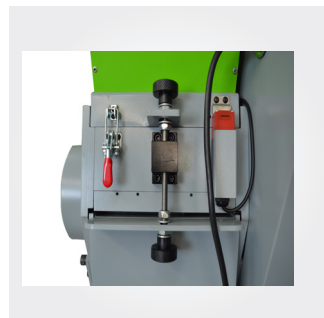
Tamper proof safety switches to prevent injury or accidental damage.
