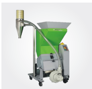
Low speed granulator shown with (optional) blower fitted.
